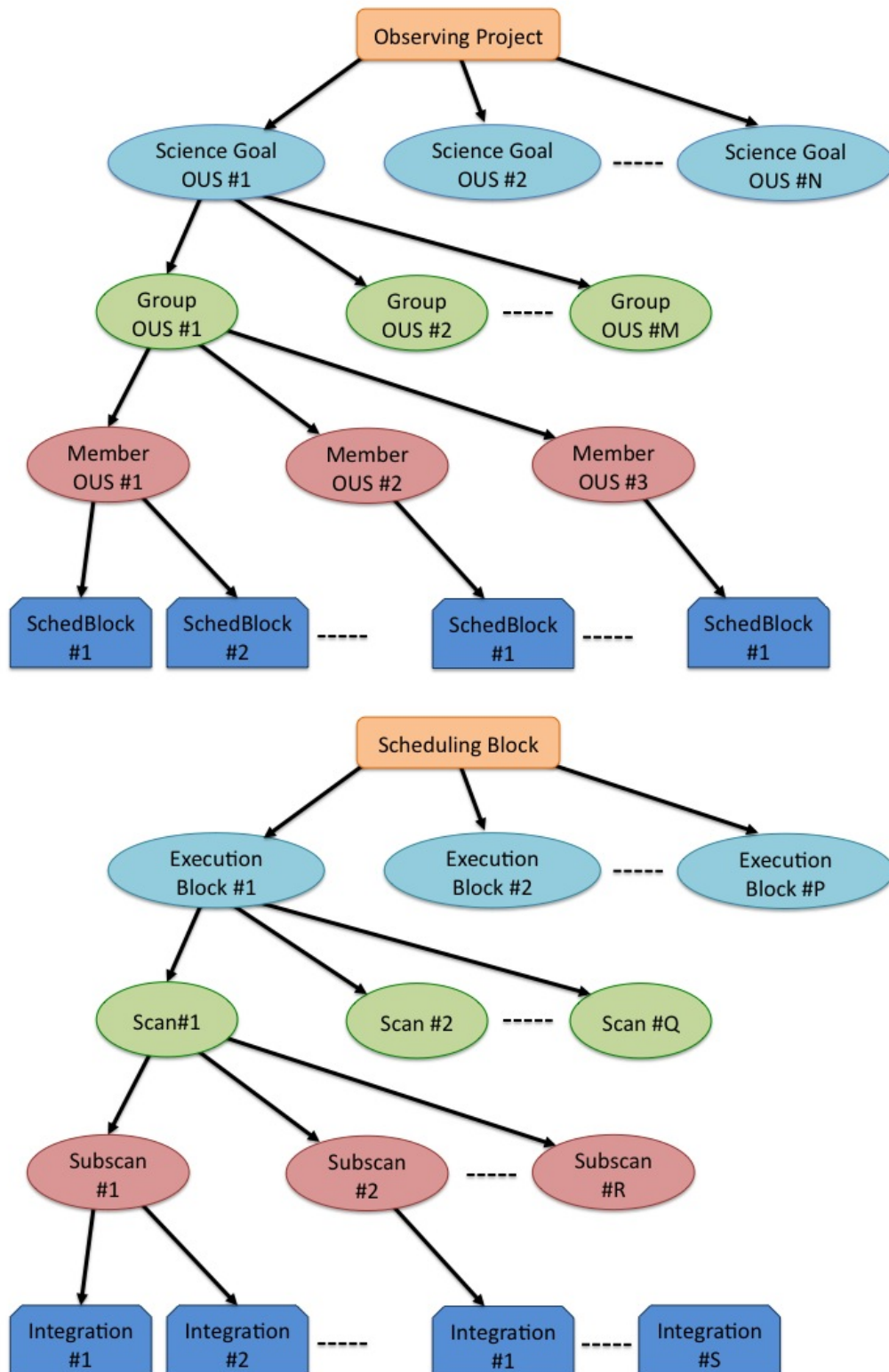
Figure 8.1: Block diagram of an Observing Project from the point of view of the observation preparation (top) and internal hierarchical structure of the SB in actual executions (bottom). All projects have the same ObsUnitSet (OUS) levels, the Science Goal OUS level, the Group OUS level and the Member OUS level. Scheduling blocks are attached to the Member OUS. Each time an Scheduling Block is executed, CONTROL creates a new ExecBlock structure (see text).
